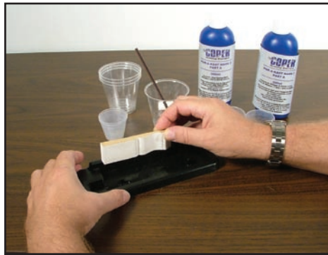
above Place the baseboard piece on edge in the casting tray- I chose to use the orientation for hardwood
