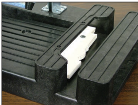
above Bolt the template into the jig
