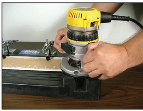
above Carefully rout the cope into the end of the baseboard
