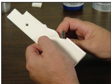
above File the template so any corners match the flush trim bit
