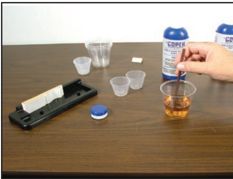
above Carefully mix the two parts together to avoid bubbles
