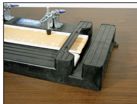
above Slide the baseboard into the jig so the end is just past the template
