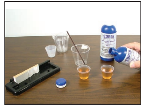
above Measure equal parts of Por-A-Kast A and B
